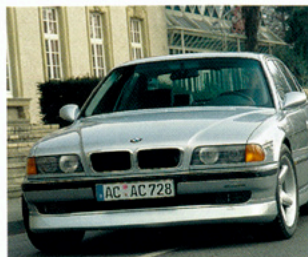
AC Schnitzer front spoiler to reduce the lift on the front axle
