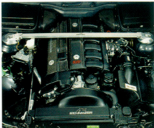
AC Schnitzer engine ACS7 3.2 for BMW 728i/iA, Performance: 191 kW (260 hp)
